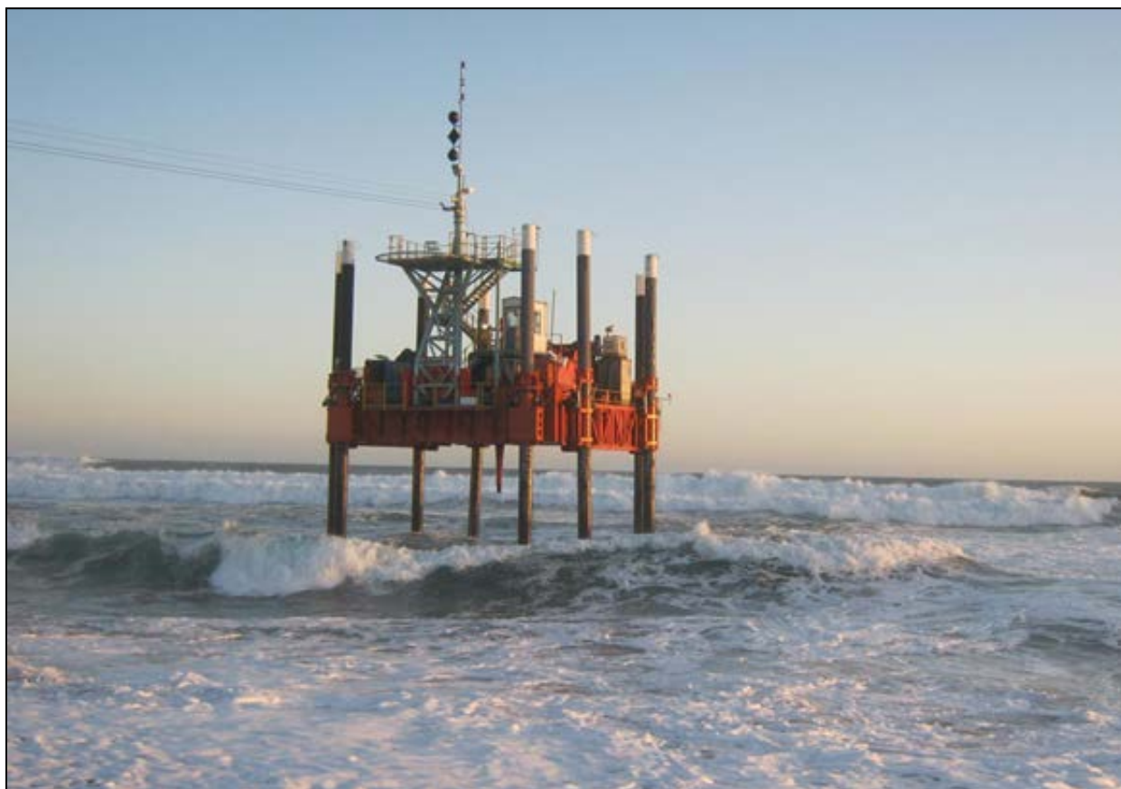
The Probe-drill Platform (PDP), a shallow marine exploration tool.
