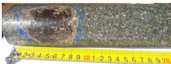
Figure 5: Core picture showing garnet harzburgite in Green coherent kimberlite from KX36 Kimberlite.
